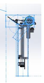
for a roller design that used very grippy Banebot wheels to actively push the gear into the deployment system. This new design not only made packaging easier it also decreased intake time thus cutting the overall cycle time.
