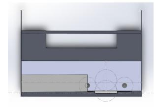
We also identified two main methods to move balls through the hopper: active and passive (gravity). We found that using gravity alone does not suffice in stopping force chains from forming. So, we developed agitators to actively move balls through the hopper.
