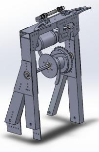
fingers which "grabs" the rope, centering it right over our drum. This would allow the drivers to have greater room for error, since the fingers would account for some misalignment, consequentially increasing the speed and reliability of our hang.
