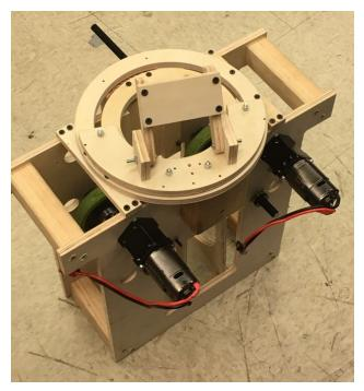
angle would also allow us to shoot from multiple positions on the field, an important factor in both autonomous programming and overall robot capability. In order to more easily package our turret, and for significantly increased shot power, we decided to shoot with 2 wheels instead of one. A 2 wheel shooter would also eliminate unnecessary spin, assuming the flywheels are spinning at relatively the same speed.
